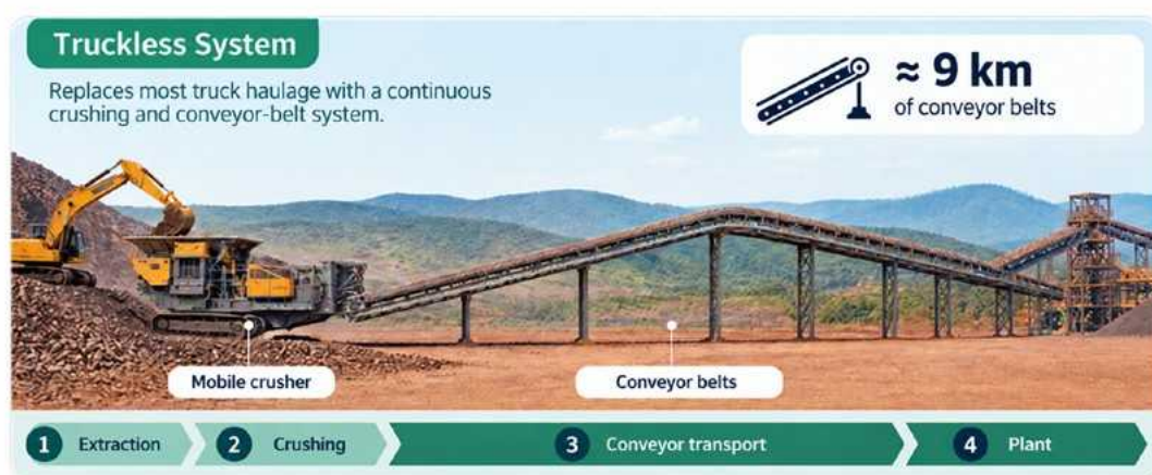
Figure 38: Operation of a truckless materials handling system
