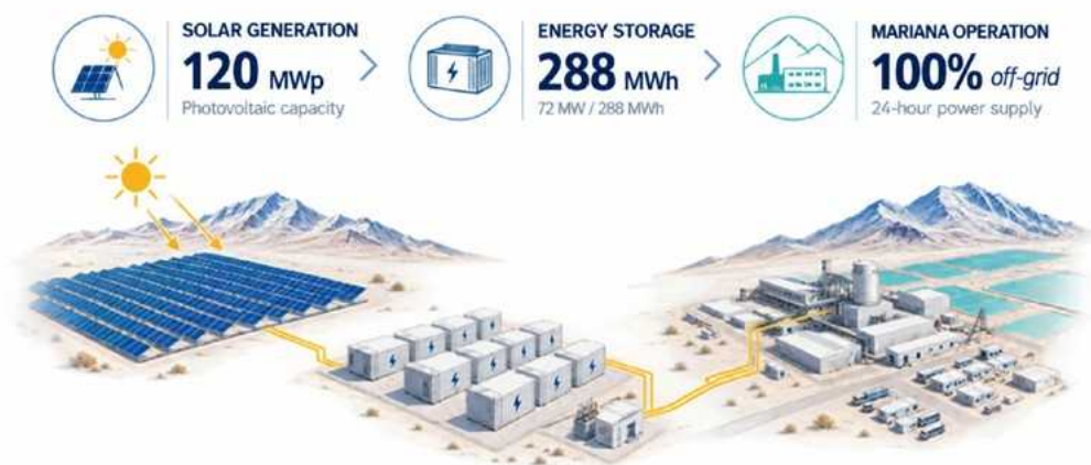
Figure 33: Off-grid renewable power system at the Mariana Project
