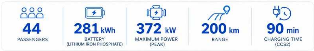
Figure 37: Technical specifications of Tricahue buses
